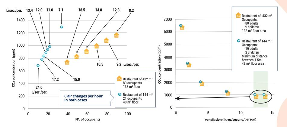
For the same dining room volume, if the number of occupants (persons) increases, the air change rate per hour should be increased to reach the recommended per person ventilation rate and avoid increase of the CO<sub>2</sub> level.
